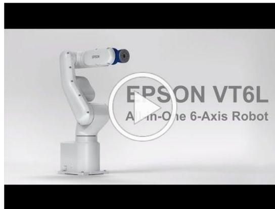
With next-level technology, the VT6L All-in-One 6-Axis robot is available at an incredible price of \$13,900, with 900 mm reach, up to 6 kg payload and built-in controller. It includes many of the features found in Epson's high-end robots, including powerful Epson RC+ development software and easy integration tools.
